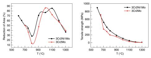
*Figure 4. Typical hot tensile mechanical properties: (left) hot ductility as a function of temperature; (right) hot tensile strength as a function of temperature.*
