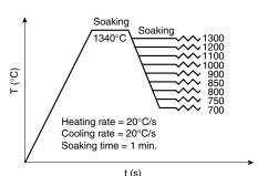
Figure 3. Test conditions of hot tensile mechanical property measurement.
