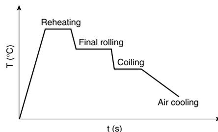
Figure 5. Thermo-mechanical processing simulation condition on the Gleeble 2000.
