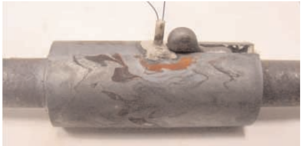
Figure 6. After simulation (shortened by axial displacement). Note excess metal ejected through the TC mounting slot.
