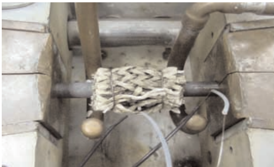
Figure 5. Setup (insulated, argon cooling jets for the ends).
